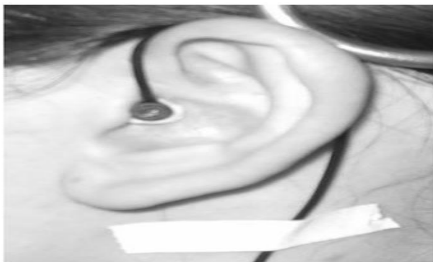
Fig.3. A Blocked Ear Canal Scheme for Microphonic Signal Data Capture [8]
